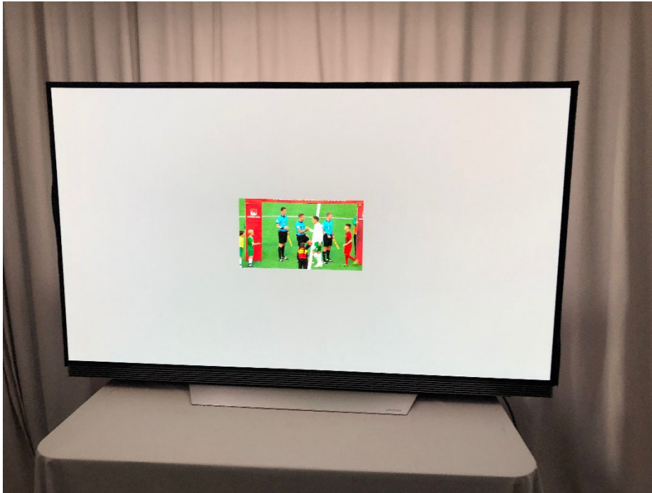
Figure 3: The video was presented in the centre of the screen with a grey surround. Here the 960x540 pixels sized video is shown.
