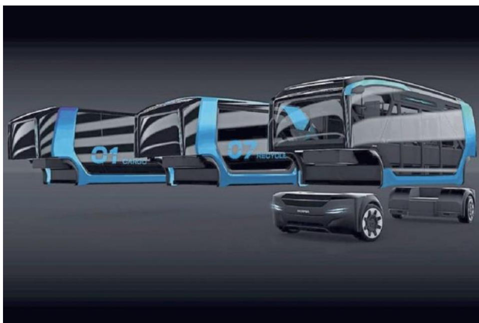
Figure 3: Scania's NXT concept. It is possible to change the bodywork to obtain a new vehicle type (e.g. from a small truck to bus), but also to change an axle. Since the axle supports the engine, the performance of the vehicle can also be altered in this way. This raises the question: what exactly constitutes the vehicle? And what kind of vehicle is it?
