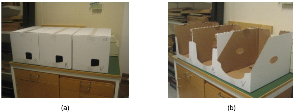
Figure 1. The perforated boxes before (a) and after (b) removal of front and top, from left to right SRP Concept A, SRP Concept B and SRP Concept C.
