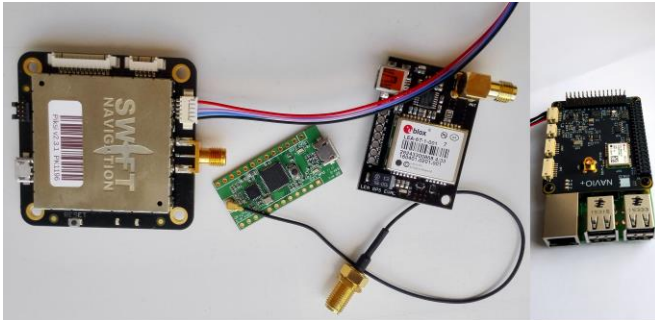
Figure 1. Evaluated GPS receivers (in order left to right, Piksi, NS-RAW, Lea-6t, Navio+)
