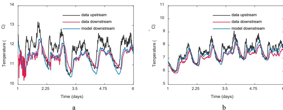
**Figure 3** Comparison between measured data and simulation results for downstream temperature from a sewer pipe for two different datasets (a. Dataset1 (Nov 2018) and b. Dataset2 (Feb 2019)) from Linköping, Sweden.
