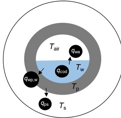
**Figure 1.** Overview of the temperature sub-model for the sewer system. Key state variables ( $T_w$ ,  $T_p$ ) and measurements ( $T_{air}$ ) are marked. Major heat fluxes considered in the temperature model are highlighted.
