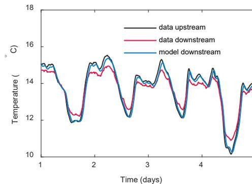
**Figure 4** Comparison between measurements and model results for the 1.5 km sewer stretch in Malmö.
