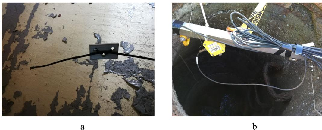
**Figure 2** (a). Thermistor probes for temperature with a weight attached to it for submerging in water and (b). Data logger connected to the thermistor probe recording temperature measurements at a pre-defined frequency of 5 minutes.
