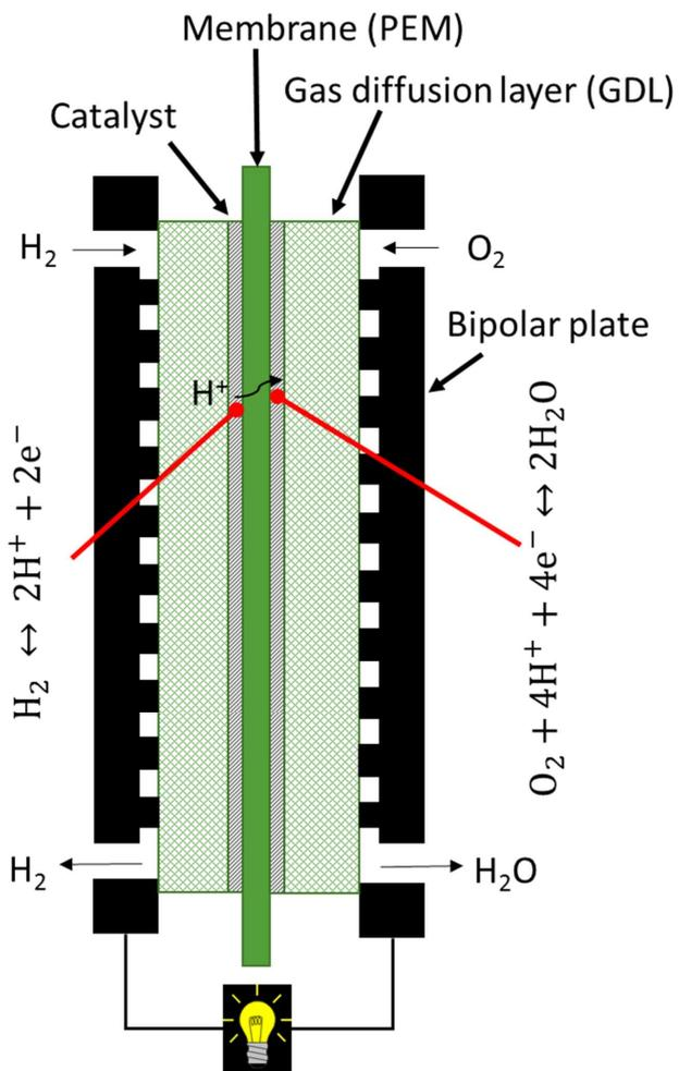
Figure 1: Sketch of the cross-section of a PEM fuel cell. Cells are stacked, making one side of the bipolar plates connected to the anode in one cell and the other side to the cathode of the next cell. Therefore, it is called a bipolar plate.
