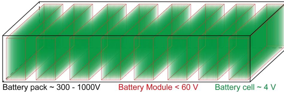
Figure 13 General construction of a battery pack.
