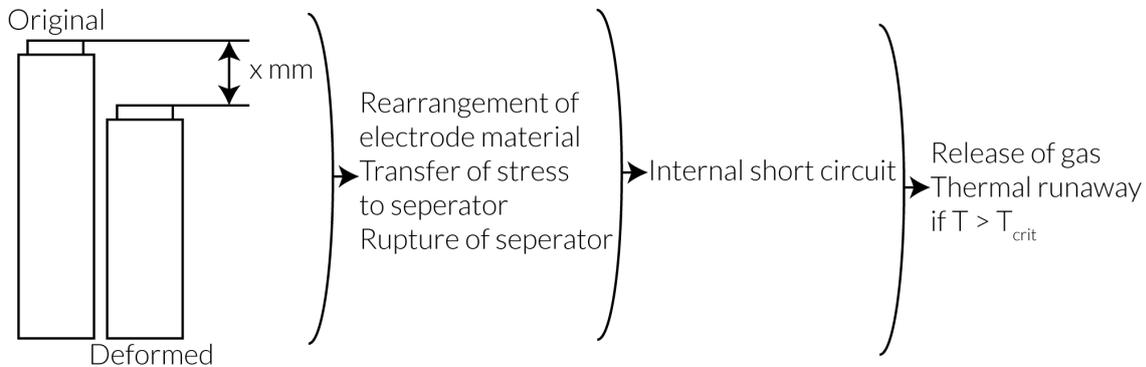
Figure 42 Mechanical deformation leading to thermal runaway [126]
