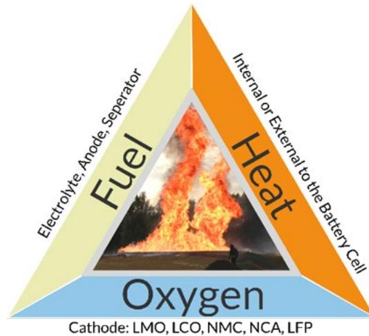
Figure 40 The fire triangle for lithium-ion batteries.
