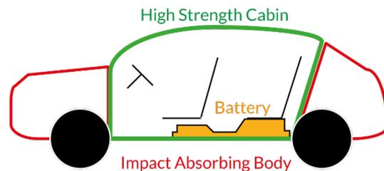
Figure 15 Battery layout for a Nissan Leaf [49]
