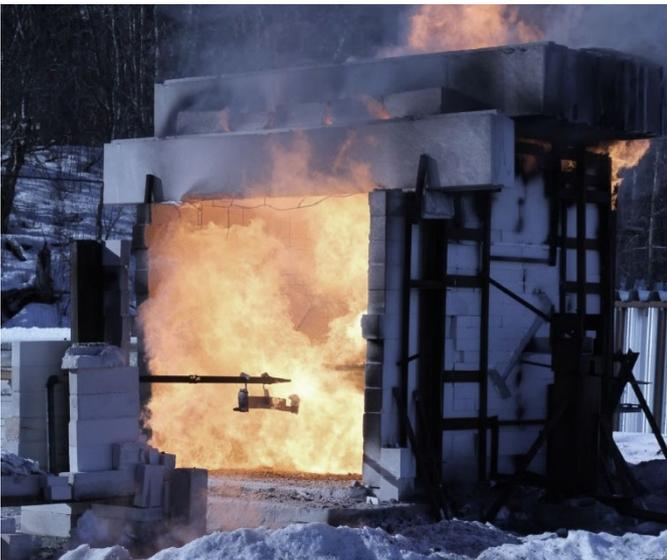
Figure B: Enlarged re-circulation chamber for high temperature jet fire testing. The bricks supporting the nozzle inlet are the same dimensions as in Figure A, enabling scale comparison.
