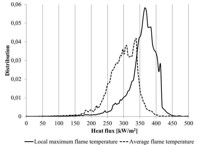
Figure F: Distribution of calculated heat flux using local maximum (solid line) and using average flame temperatures (dashed line). Data is collected from 55 high temperature jet fire tests, each with about 6 thermocouples.
