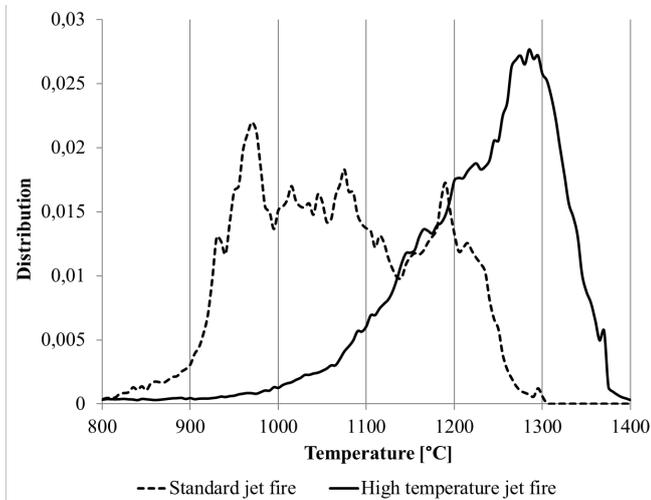
Figure E: Flame temperature measurement distribution in jet fire tests. Data from a total of 20 standard jet fire tests, with average temperature  $1061 \pm 115^\circ\text{C}$ , median  $1059^\circ\text{C}$  (dashed line). Data from a total of 55 high temperature jet fire tests, with average temperature  $1218 \pm 179^\circ\text{C}$ , median  $1244^\circ\text{C}$  (solid line). All temperature measurements at each recorded time step are included in the data set.
