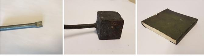
Figure C: Thermocouple systems used in jet fire tests. Tube thermocouple (left), cube thermocouple (center) and plate thermocouple (right).
