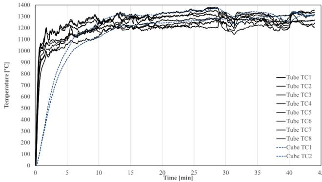
Figure D: Flame temperatures measured using tube and cube thermocouples (TC) in one high temperature jet fire test. Solid lines indicate measurement by tube thermocouples, dashed lines indicate use of cube thermocouples.
