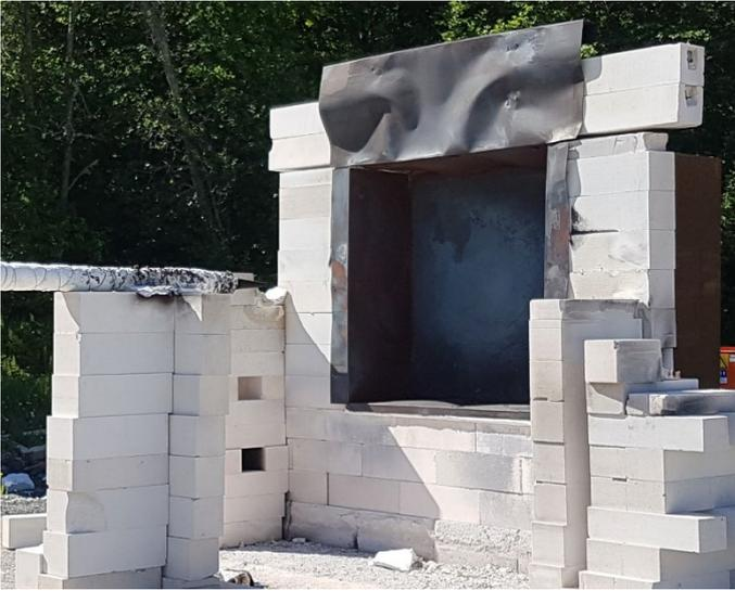
Figure A: Design of the re-circulation chamber according to ISO 22899-1 [2].
