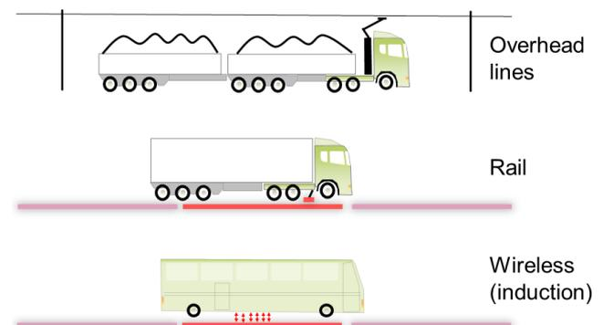
Fig. 1 The three main concepts for road electrification and electric power transfer to moving vehicles.
