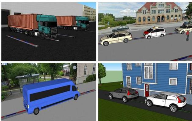
Fig. 2 Examples of applications utilizing road electrification by means of a rail solution. Pictures courtesy of Dan Zethraeus.
