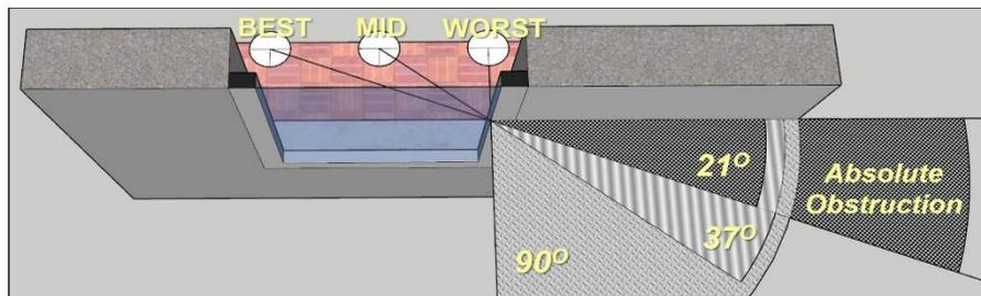
Figure 6 Three different viewing positions have different possibilities for width of view.
