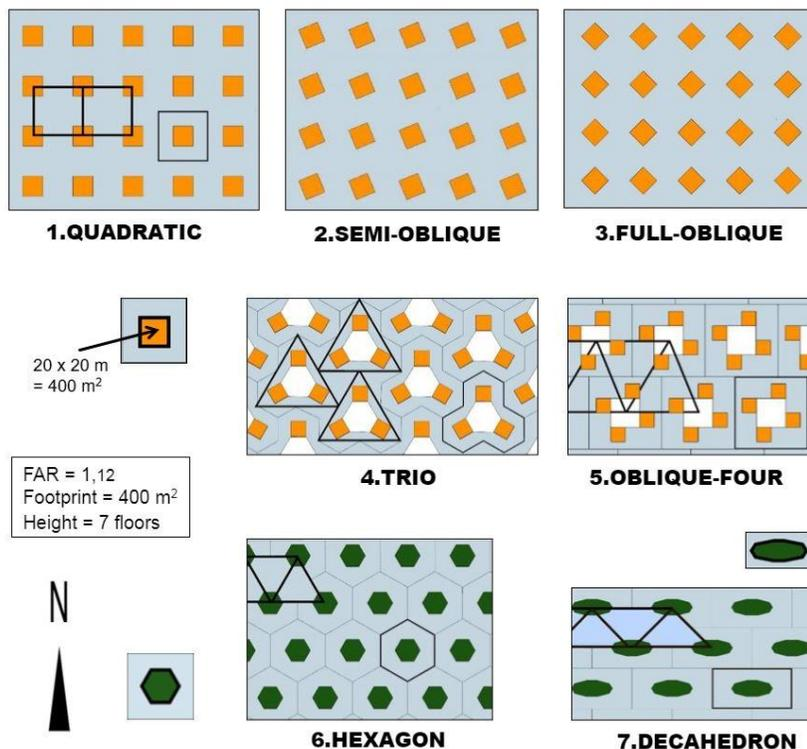
Figure 3 The seven alternatives for groups of tower blocks.
