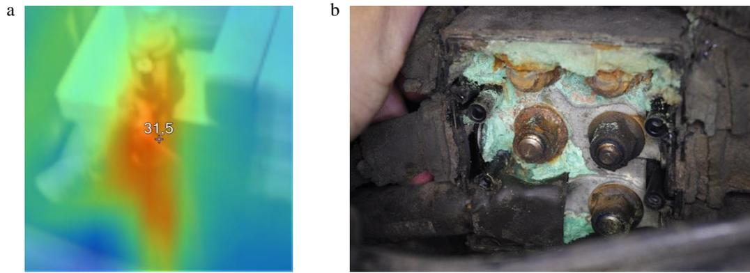
Fig. 2 (a) Thermal image of the positive terminal of a car battery which indicates a poor connection, marker displays degrees Celsius; (b) Oxides in a terminal block detected by a thermal imaging camera
