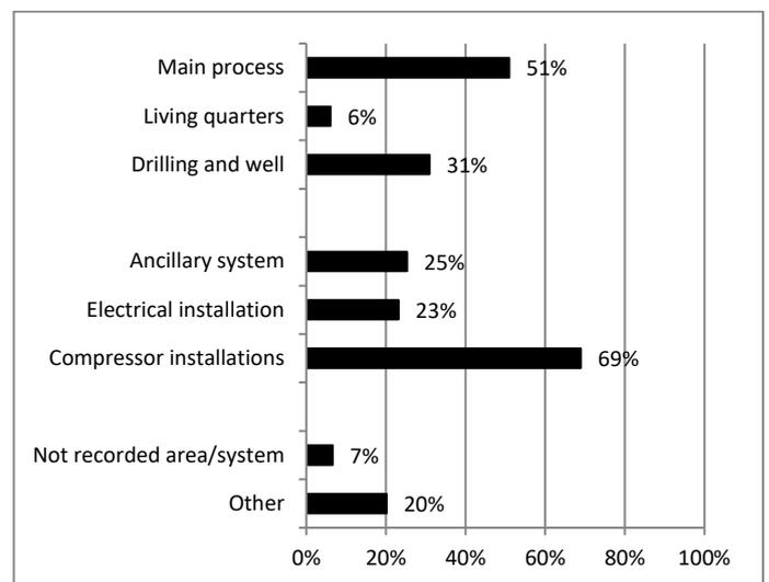
**Figure 6** Incidents causing production stoppage distributed over the area or system the incident occurred in. Areas and systems with fewer than 20 reported incidents are excluded from the figure, n = 231.
