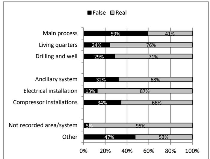
Figure 10 Proportion of real and false alarms for each area and system. Areas and systems with fewer than 20 reported incidents are excluded from the figure. Main process n = 102, living quarters n = 66, drilling and well n = 42, ancillary system n = 305, electrical installations n = 95, compressor installations n = 29, not recorded n = 182, other n = 139, total n = 960.
