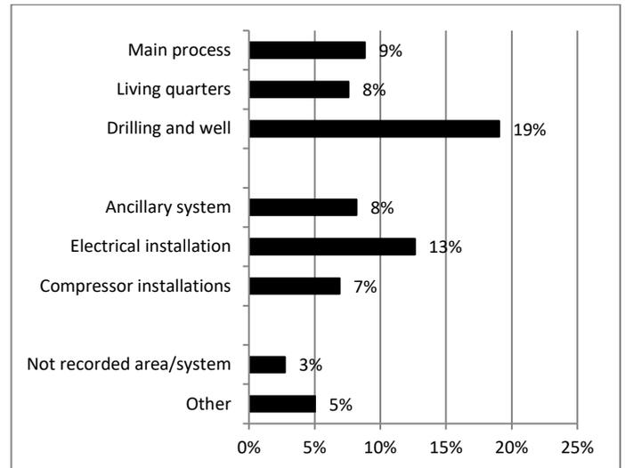
**Figure 5** Incidents causing drilling downtime, distributed over the area or system the incident occurred in. Areas and systems with fewer than 20 reported incidents are excluded from the figure, n = 76.
