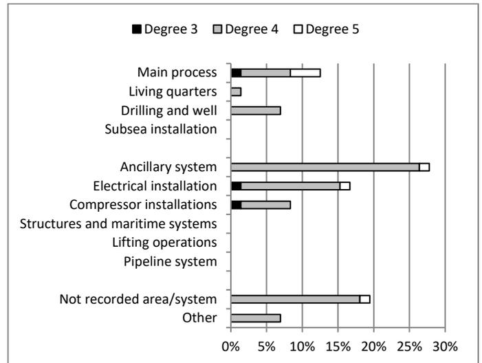
**Figure 7 Incidents with severity degree 3 (n=3), 4 (n=63) or 5 (n=6), distributed over different areas and systems, total n = 72.**
