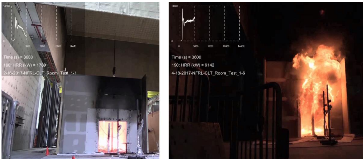
Figure 3: Fully encapsulated compartment (left) and compartment with an exposed CLT wall and ceiling (right) 1 hour after ignition (Frame of a video by NIST, USA).
