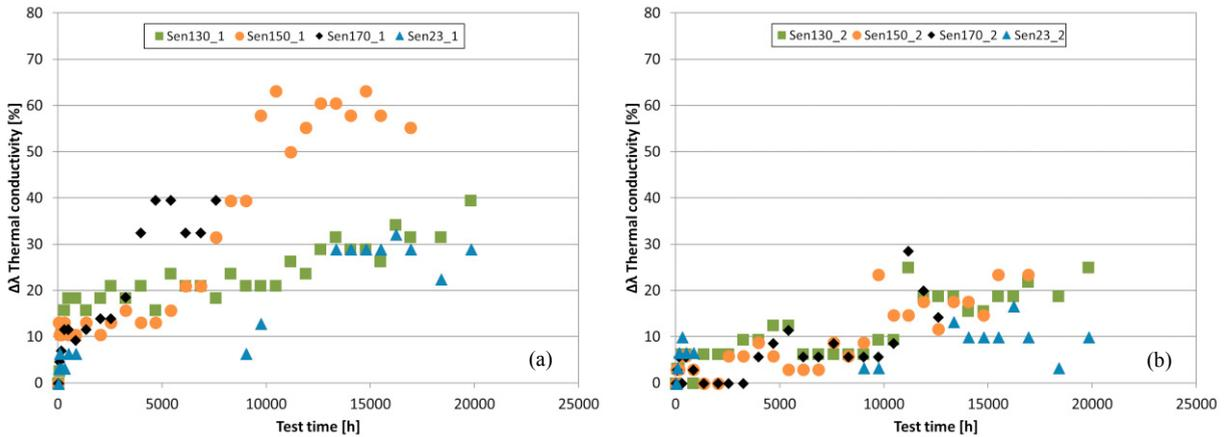
Fig. 2. Thermal conductivity measurements. (a)  $\Delta\lambda$  measured by the sensor positioned at 5 mm and (b) 30 mm in each pipe.
