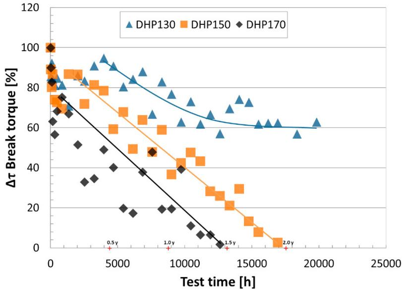
Fig. 1. Mechanical shear strength measured by the SP plug method.
