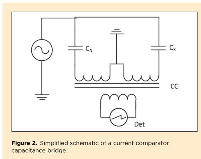
Figure 2. Simplified schematic of a current comparator capacitance bridge.
