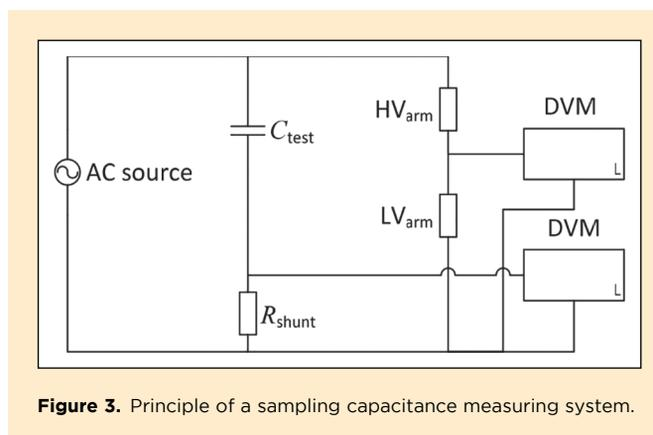
Figure 3. Principle of a sampling capacitance measuring system.
