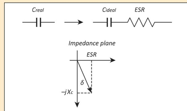
**Figure 4.** Relation between equivalent series resistance ESR and capacitance.
