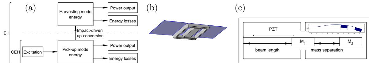
**Figure 1.** (a) The impact and cantilever EH approaches. (b) A conceptual double bridge IEH. (c) The double cantilever EH. The inset shows the harvester (second) mode.
