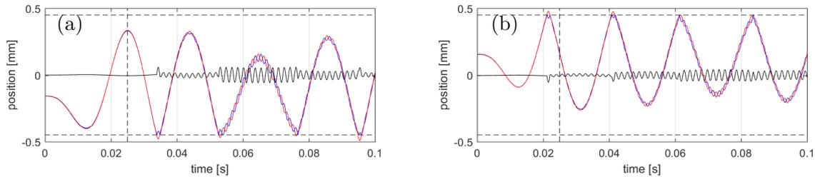
**Figure 2.** The position of  $M_1$  (blue),  $M_2$  (red), and their separation (black). The dashed lines indicate the position of the capping and the end of the excitation. (a) Gravity acts downwards and impact occurs after the end of the excitation. (b) Gravity acts upwards. The earlier impact reduces the system energy.
