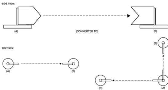
**Fig. 4.** The side view shows how to aim the Nodes to connect device A to device B. The top view shows two networks: one in which device A is connected to device B, and another in which A is connected to both devices B and C.
