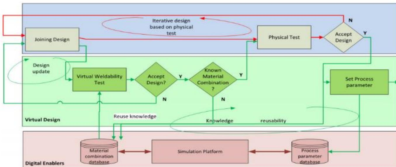
Fig.1. Process flow and digital enablers to implement virtual testing in RSW process [2]
