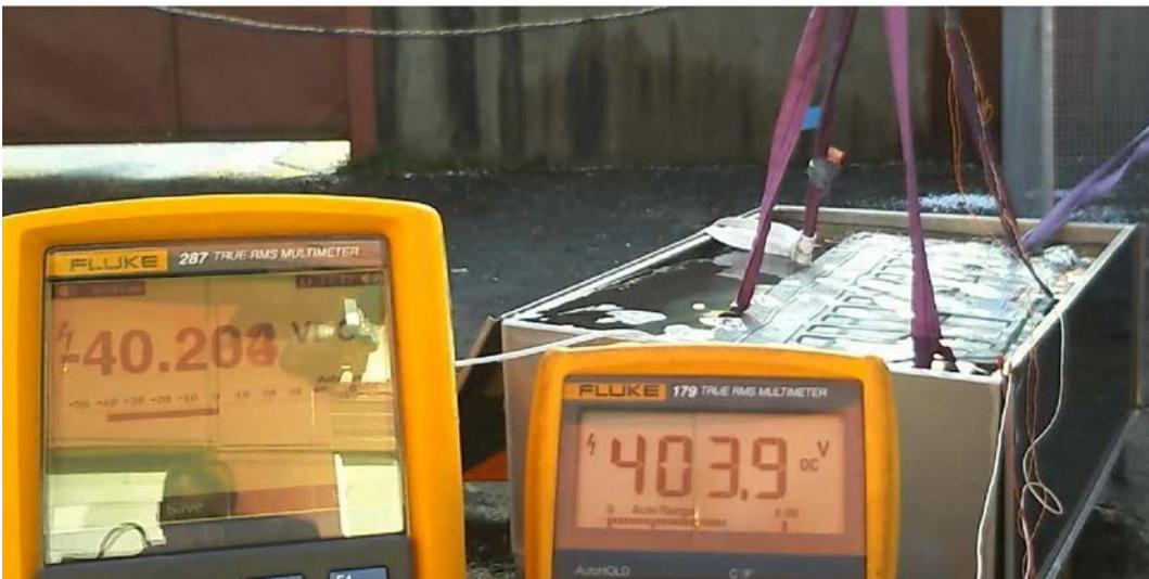
Figure 5, The battery's inbuilt system opens the main contactors immediately, the measurement instrument to the left is connected after the main contactors and the instrument to the right, before this.
