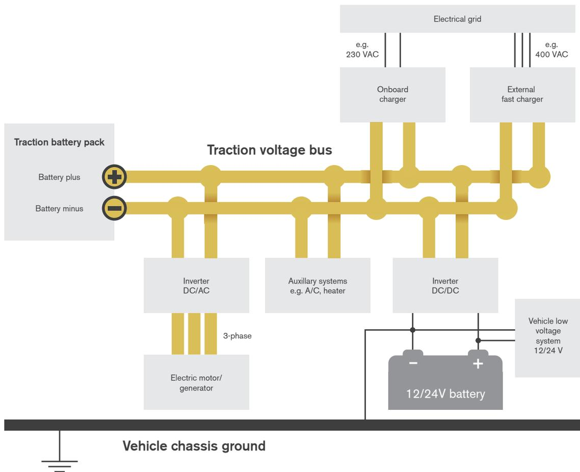
**Figure 4.3.** Schematic overview of a traction voltage system in an electrified vehicle connected to the electrical grid. The traction voltage bus (with DC voltage) with floating ground principle is shown.
