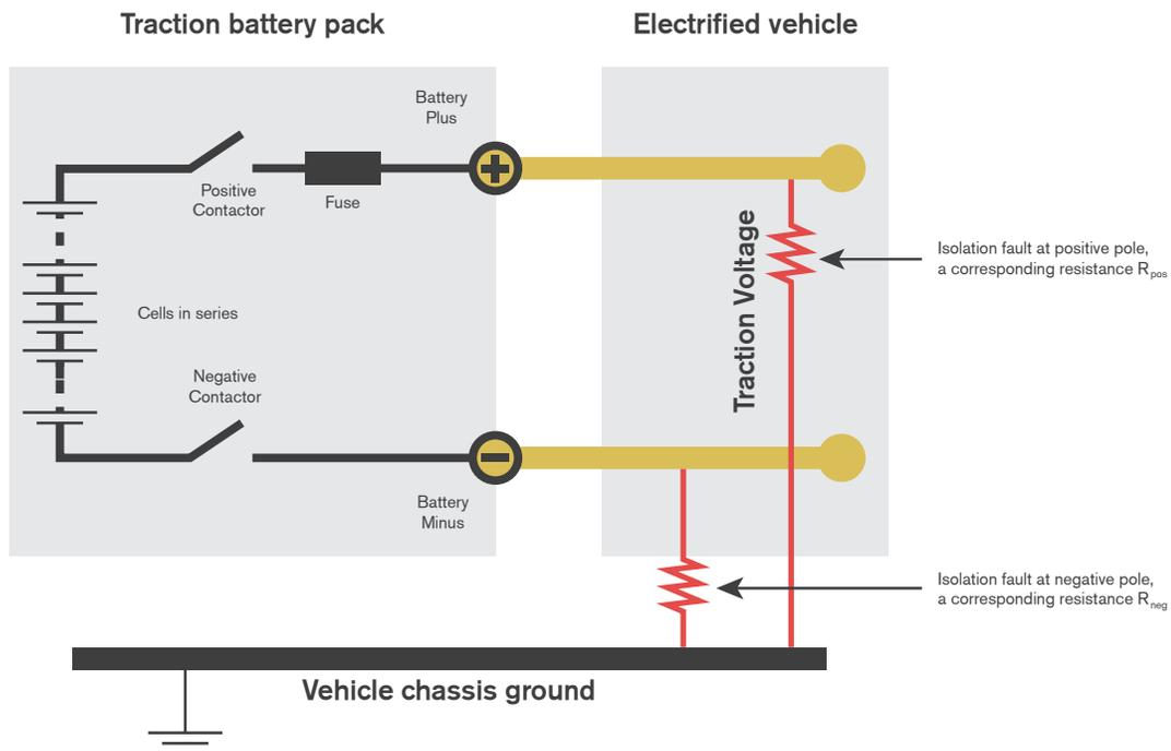
**Figure 4.5.** Principle figure that shows a double insulation fault. This means one insulation fault at the plus and one at the minus pole. They are shown as two resistances,  $R_{pos}$  and  $R_{neg}$ , connected to ground. This creates a current path between battery plus and battery minus through the vehicle chassis ground.
