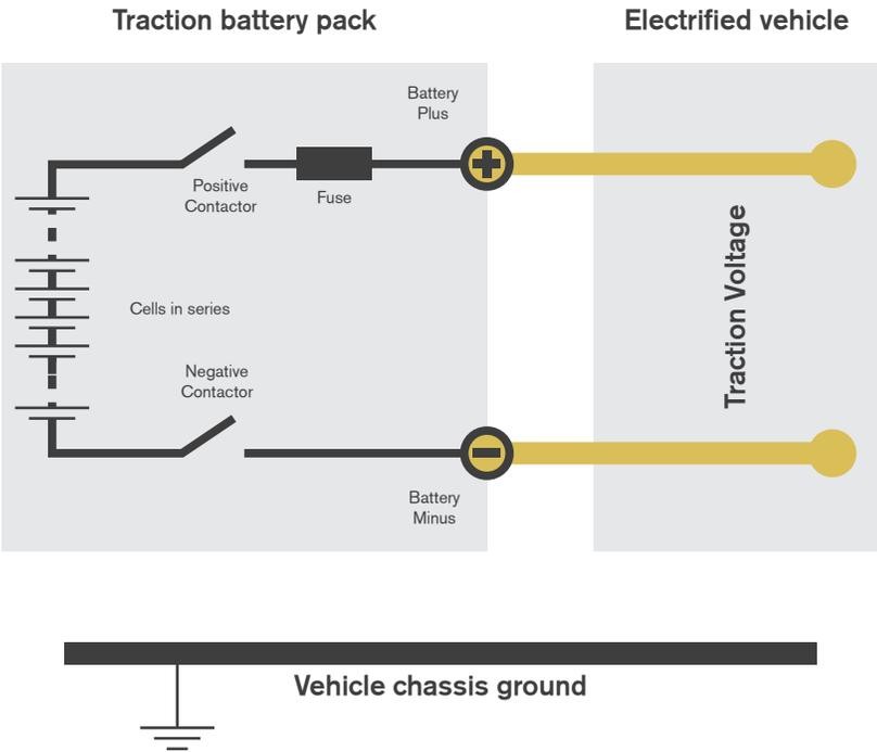
**Figure 4.4.** Traction battery pack current path and the floating ground principle. If there are no insulation fault(s), there are no electrical connections between vehicle chassis ground and the battery poles.
