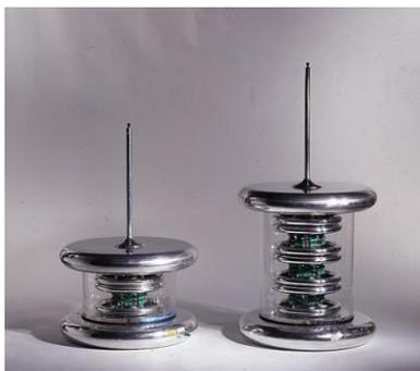
Figure 3: Vishay DC reference voltage dividers for 50 and 100 kV
