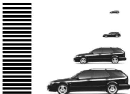
**Fig. 1** The principle behind the Johnson criteria, being based on the number of cycles, shown by the bar pattern to the left at a distance, where it will be just resolvable (about 3 m). The images to the right representing detection, orientation, recognition, and identification, where the height of each image corresponds to a number of cycles in the bar pattern.
