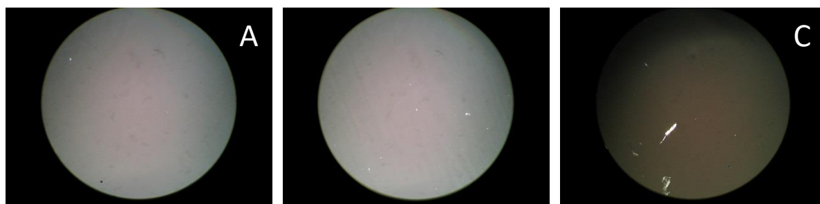
Figure 2. Images of cellulose solutions of (A) 5 wt% P2, (B) 5 wt% P3 and (C) 7.5 wt% P1, obtained by cross-polarized microscopy.
