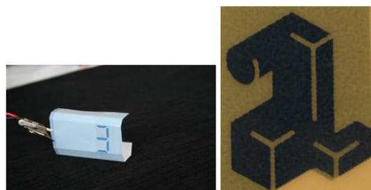
**Figure 3.** Left: a lateral 7-segment ECD manufactured by roll to roll printing on top of a paper substrate is shown. Right: the photograph shows the colored state of a vertical ECD upon applying 3V. The display pattern resembles the logotype of Acreeo.
