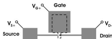
**Figure 4.** The architecture of a lateral ECT is shown. A vertical ECT device is obtained by simply stacking the gate electrode on top of the transistor channel with the electrolyte layer sandwiched in between.
