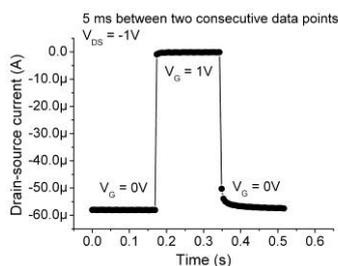
**Figure 6.** The switching characteristic of a printed ECT is shown, wherein each switching event occurs in less than 5 ms.
