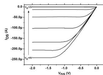
**Figure 5.** The current through the transistor channel is recorded while sweeping the voltage between the drain and source electrodes. Each voltage sweep corresponds to a certain gate voltage.
