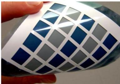
**Figure 7.** The photograph shows an active-matrix display containing 5×5 smart pixels.
