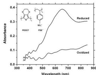
**Figure 1.** The chemical structures of PEDOT and PSS are illustrated. PSS maintains charge neutrality when PEDOT is oxidized, and  $\text{Na}^+$  is typically used as the cation. An electrolyte based on PSSNa has also been used in many of the presented components herein. The upper and lower graph represents the reduced blue-colored and the oxidized white-colored state, respectively.
