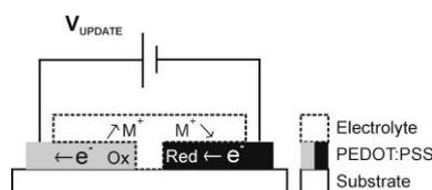
**Figure 2.** The architecture of a lateral ECD is shown. A vertical display device is obtained by simply stacking the electrodes on top of each other with the electrolyte layer sandwiched in between.
