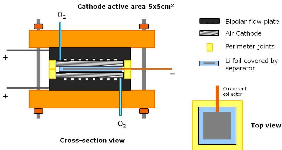
*Figure 2 Working prototype lithium-air cell*
