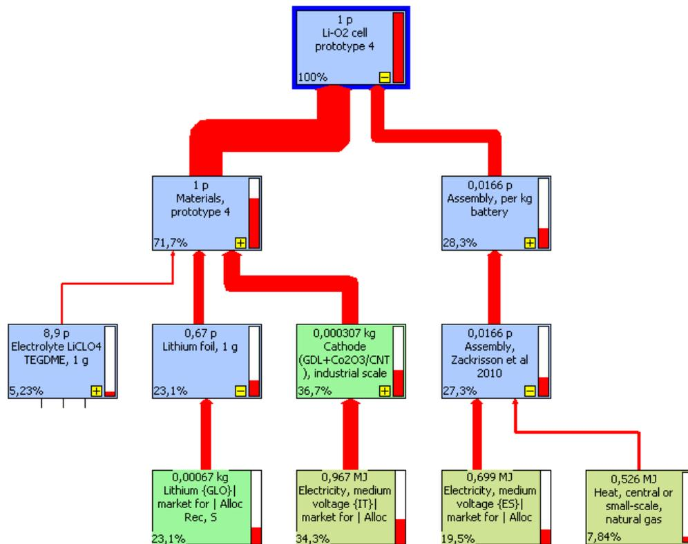
Figure 4 Relative climate impact of cell components
