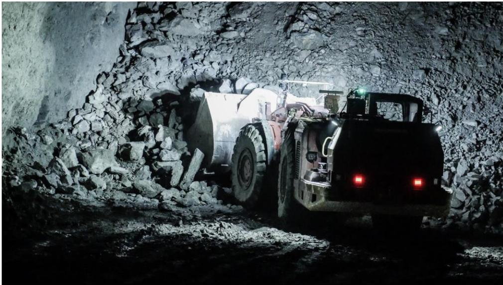
Fig 3. The remote controlled LHD.
