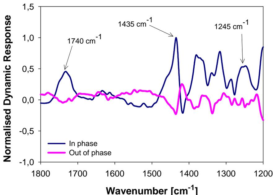
**Fig. 4.** Dynamic FTIR spectrum of oriented sheets of aspen holocellulose recorded at 0% RH, 30 °C, 0° polarization. The sinusoidal stretching was applied transverse to the fiber direction.
