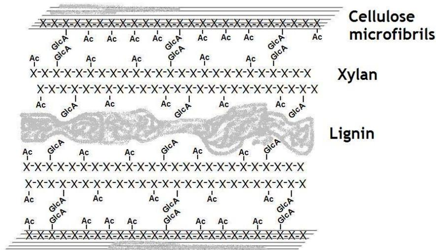
**Fig. 5.** Schematic picture of a proposed model for the arrangement of cellulose, xylan and lignin in the secondary cell walls of aspen wood. Note that the xylan has been greatly enlarged for better illustration. Gray areas represent lignin.
