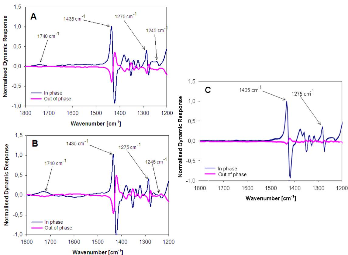
**Fig. 2.** Dynamic FTIR spectrum of water-extracted nanocomposite recorded at (A) 0% RH and (B) 85% RH, and for (C) bacterial cellulose recorded at 0% RH.  $T = 30\text{ }^{\circ}\text{C}$ . In all cases the IR-irradiation used was of  $0^{\circ}$  polarization.
