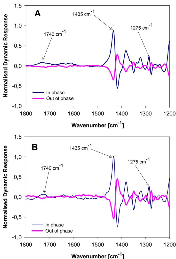
**Fig. 3.** Dynamic FTIR spectrum of oriented sheets of aspen holocellulose recorded at 0% RH, 30 °C, 0° polarization (A) and 85% RH, 30 °C, 0° polarization (B). The sinusoidal stretching was applied in the fiber direction.
