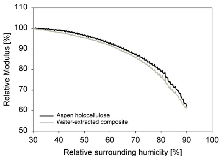
**Fig. 1.** Softening behavior of the aspen holocellulose and water-extracted nanocomposite as a function of surrounding relative humidity at 30 °C.
