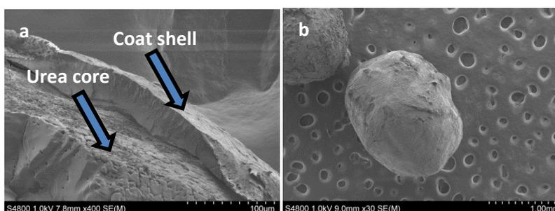
**Figure 1.** SEM images of a PLA-functionalised lignin complex-coated urea pellet, showing a coating layer over urea core (a) and outlook of a coated pellet (b)
