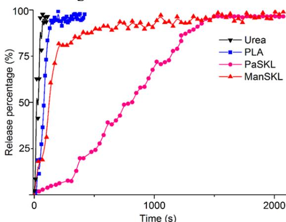
**Figure 2.** Results of the circulating water release test for urea release percentage from coated urea pellets after determination using UV at 200 nm. The release percentage was relative to the highest possible reading.
