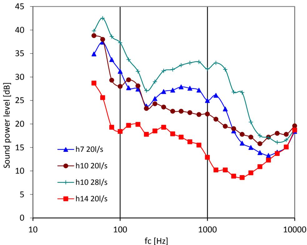
Figure 8 ATD third octave band sound power levels
