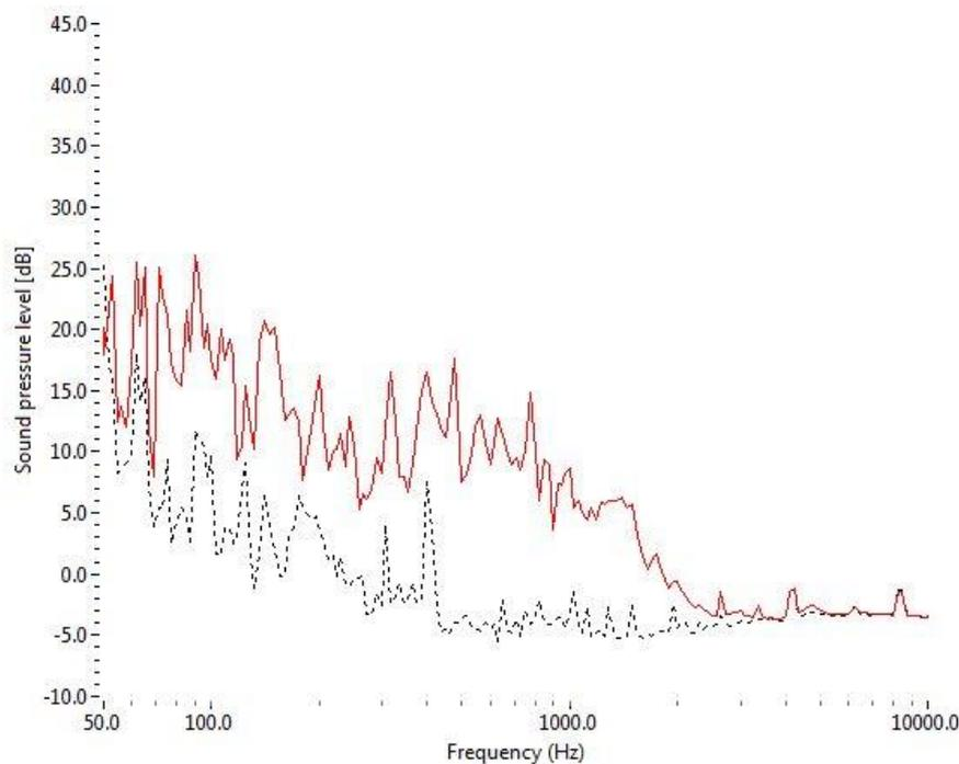
Figure 9. Sound pressure level in receiving room for standard case (red line) i.e. HRU airflow 70 l/s and ATD h10 airflow 20 l/s using a 600 mm long silencer. Background level (dashed black line)
