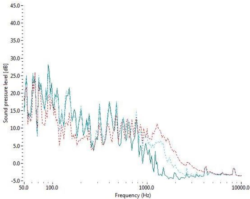
Figure 10. ATD with different settings; h14 (green), h10 (dashed light blue), h7 in combination with HRU silencers (dashed red)
