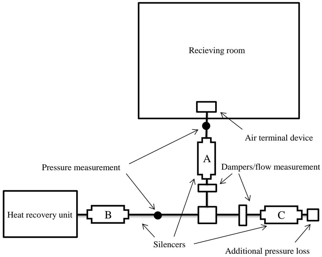
Figure 4. Layout of the HVAC system setup
