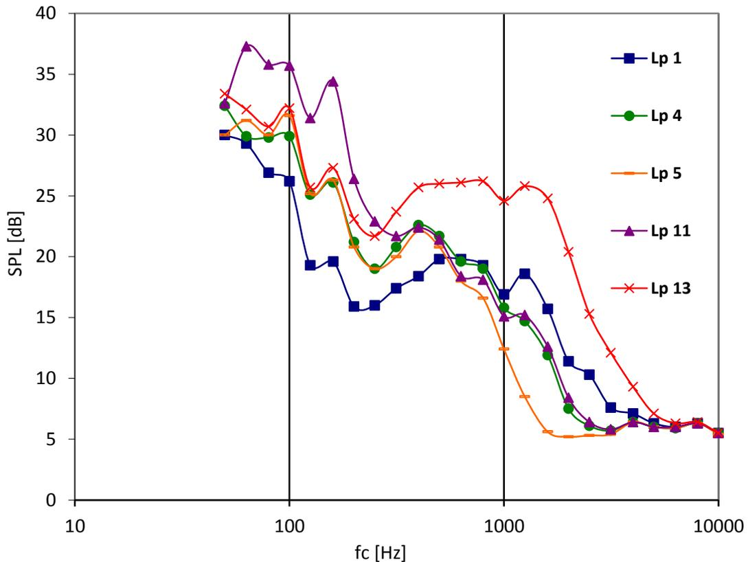
Figure 12. Third octave band sound pressure levels for HVAC system setup where ATD settings are: h7 (Lp1), h10 (Lp4), h14 (Lp5), h7 and HRU at high airflow (Lp11), h10 and ATD at high airflow (Lp13)
