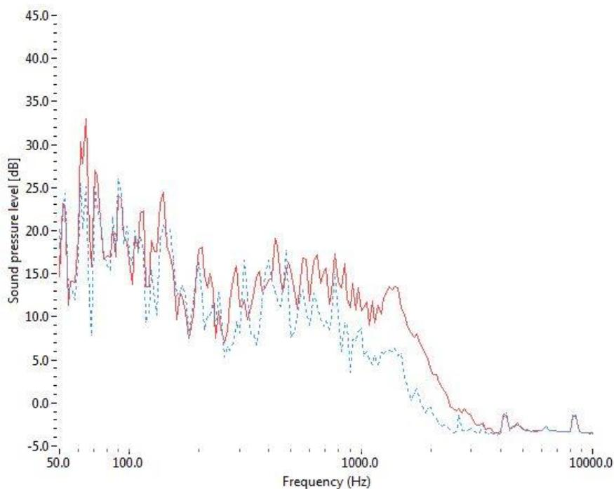
Figure 11. Bend before ATD at an airflow of 20 l/s: h10 (dashed light blue) and bend next to ATD h10 (red)
