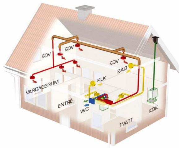
Figure 1. Common HVAC system layout in residential buildings. Picture used with permission from Fläkt Woods
