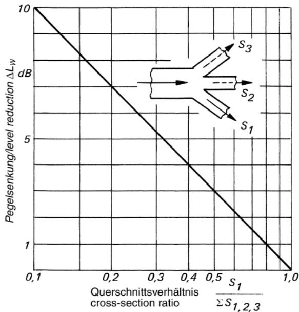
Figure 2. Level reduction at junctions. Picture from VDI 2081
