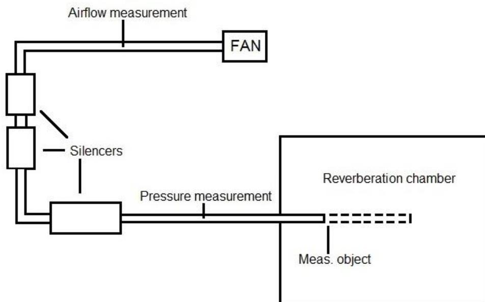
Figure 7. Measurement setup for airflow, static pressure drop and sound power measurements
