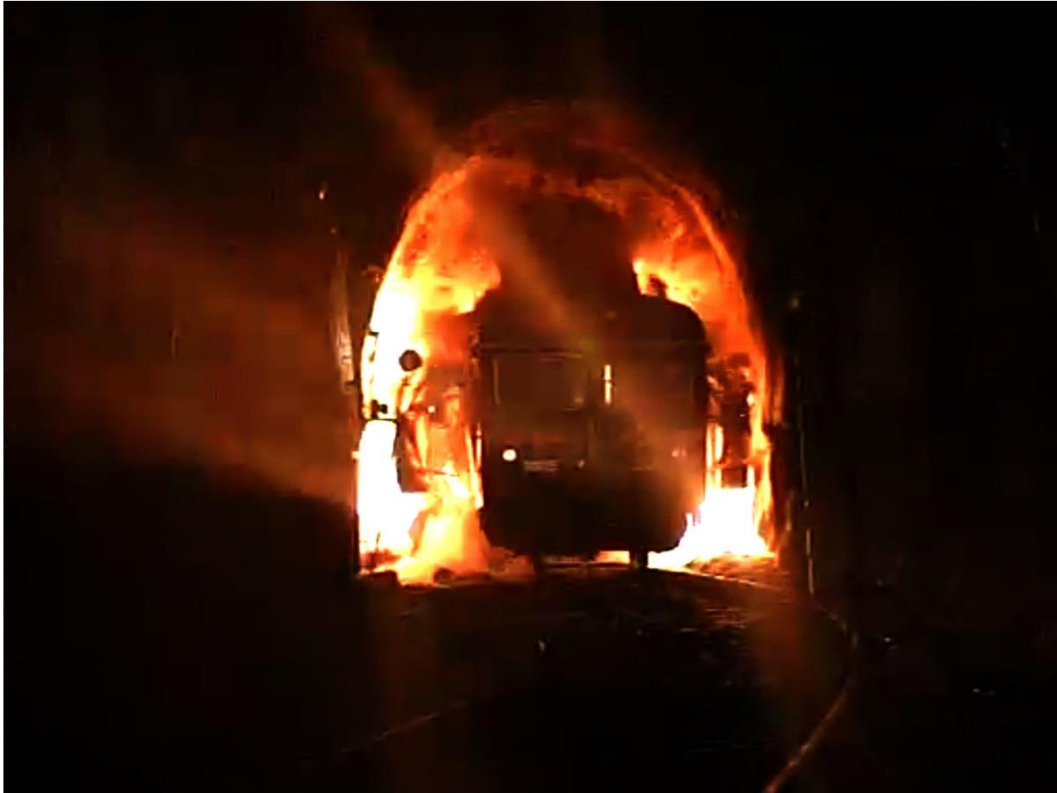
Figure 2 : A photograph of an explosion in a train carriage, taken during the 'METRO' project (FOI).
