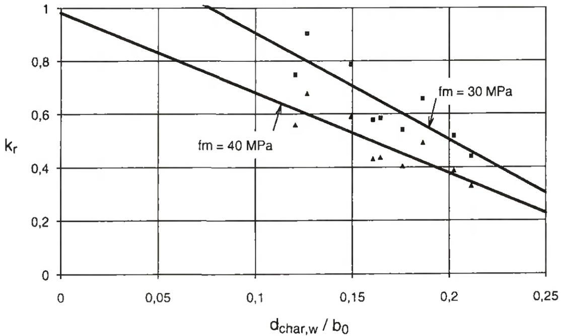
**Figure 7** Bending strength ratio of residual cross section versus relative charring depth
