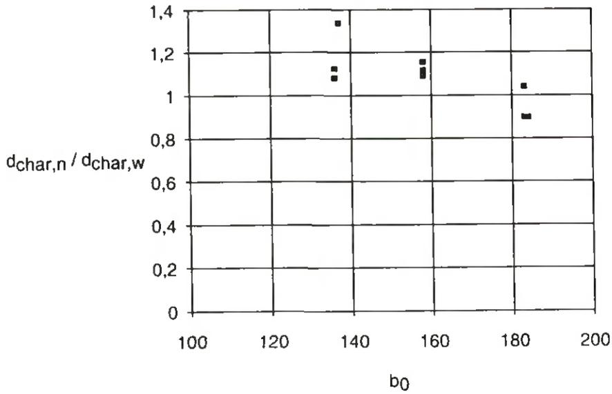
**Figure 6** Ratio of charring depths on narrow and wide side versus initial width of narrow side
