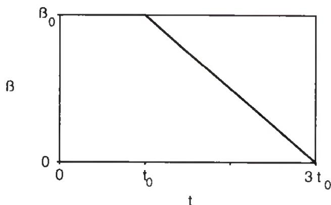
Figure 1 Simplified relationship between charring rate and time
