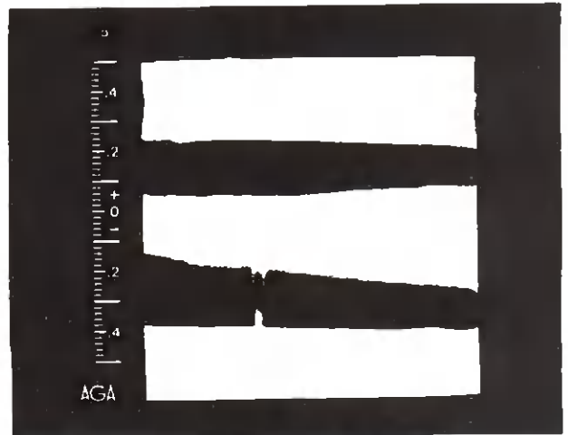
Figure 3: Thermography of wooden surfaces. Dark areas mean a lower temperature than light areas. Top: 7 minutes after start. In the heartwood the earlywood temperature is about 2°C lower than the temperature in the latewood. Bottom: 62 minutes after start. The temperature of the sapwood is about 5°C lower than the heartwood temperature.
