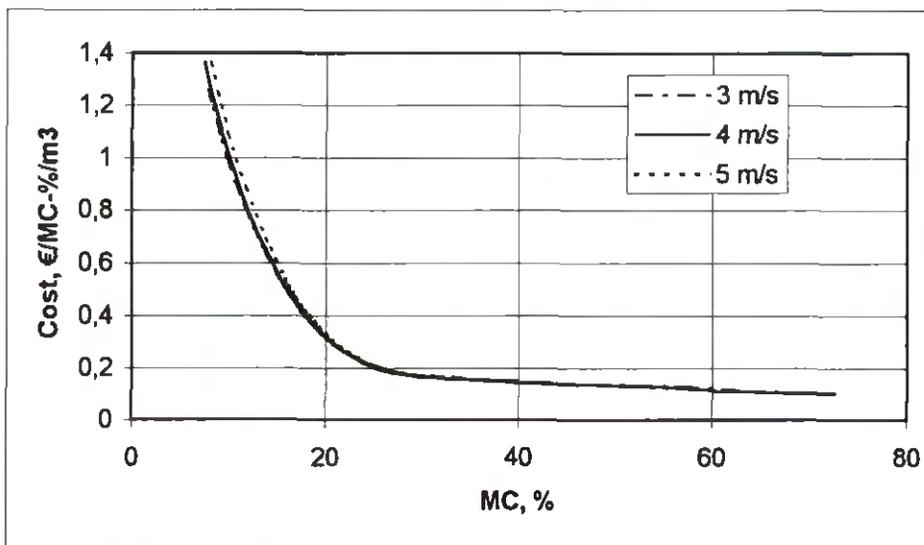
Figure 4. Instantaneous total cost for different air velocities. Maximal temperature 80°C.
