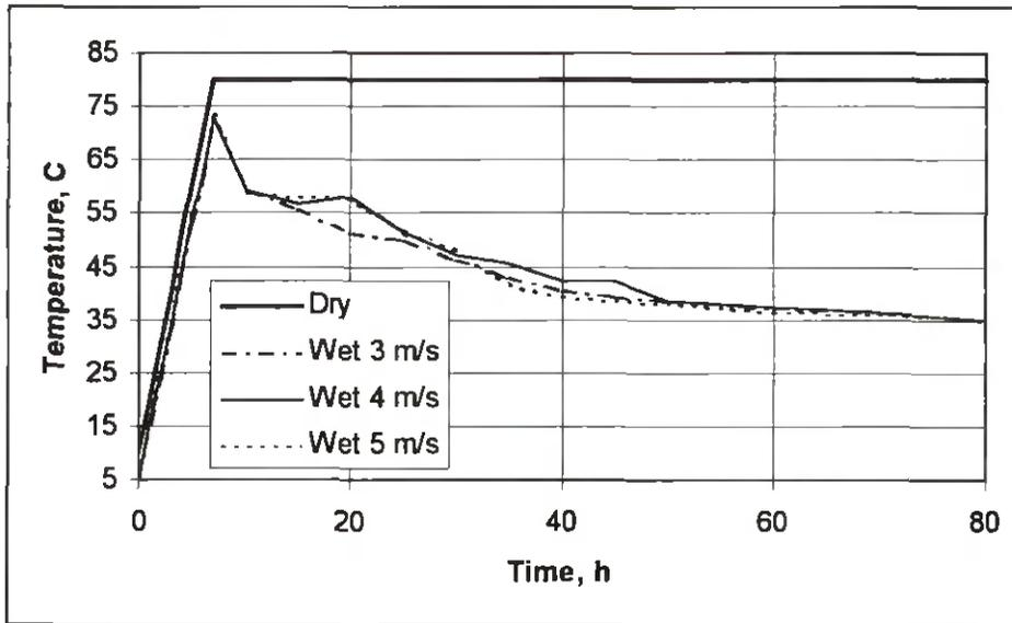
Figure 3. Optimal drying schedules for different air velocities. Maximal temperature 80°C.
