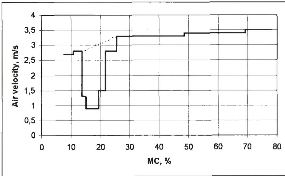
Figure 8. Optimal cost air velocity. Maximal temperature 60°C.
