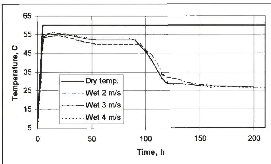
Figure 5. Optimal drying schedules for different air velocities. Maximal temperature 60°C.
