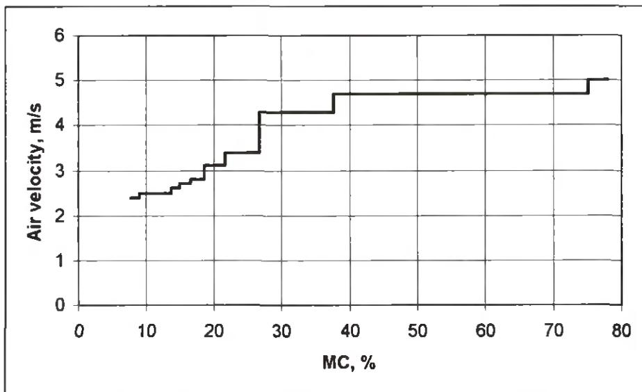
Figure 7. Optimal cost air velocity. Maximal temperature 80°C.
