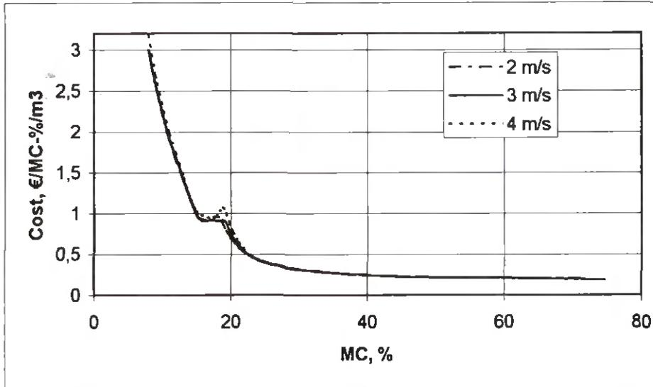
Figure 6. Instantaneous total cost for different air velocities. Maximal temperature 60°C.
