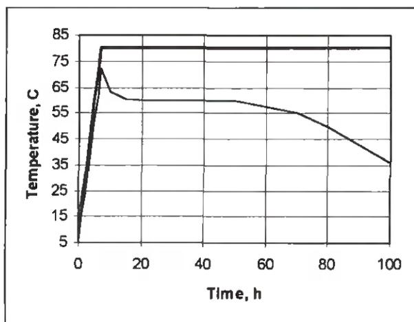
FIGURE 3. Dry and wet bulb temperature drying schedule for the numerical case studied.
