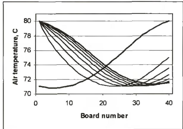
FIGURE 7. Air temperature profiles in the stack centre part during one fan reversal cycle.
