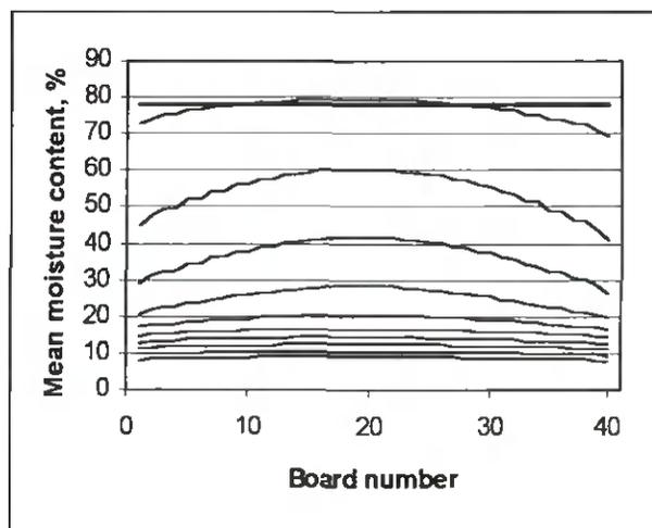
FIGURE 5. Board moisture profiles in the airflow direction in the stack end parts (10 h between curves).
