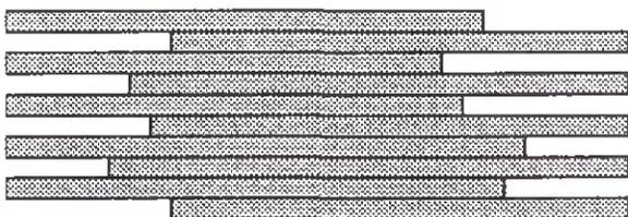
FIGURE 1. Layer of random length boards seen from above.
