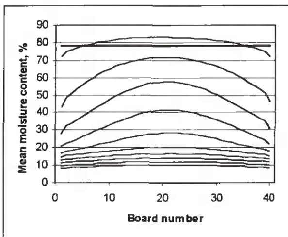
FIGURE 4. Board moisture profiles in the airflow direction in the stack centre part (10 h between curves).
