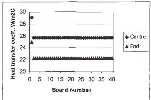
FIGURE 2. Heat transfer coefficients for the centre and end part of individual boards. Air velocity is 3 m/s between board layers in the centre part.
