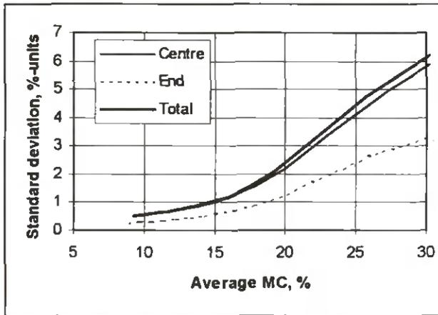
FIGURE 6. Board MC standard deviation as a function of average MC.
