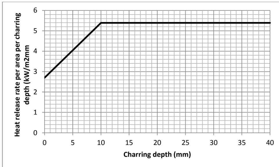
Figure 3-5: Heat release rate per unit area per charring depth
