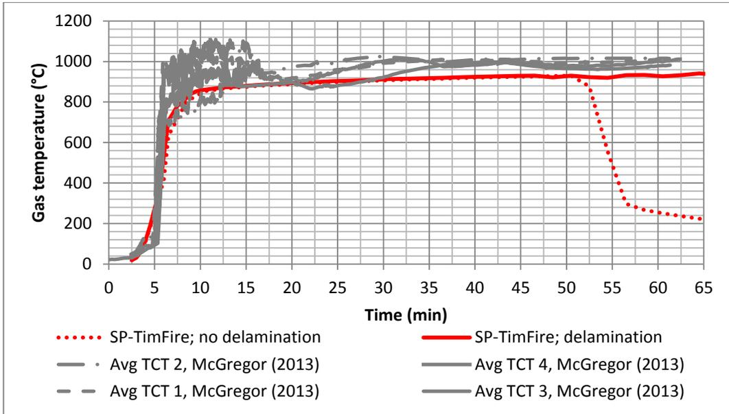
Figure 4-2: Experimentally determined and predicted temperatures for a compartment with exposed CLT walls and ceiling according to SP-TimFire
