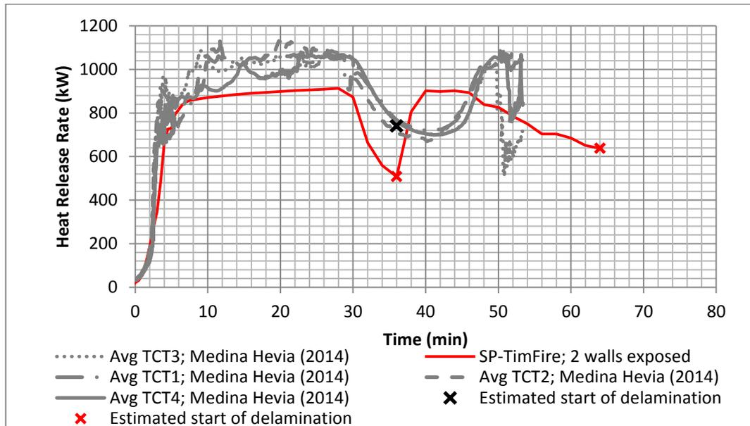
Figure 4-4: Experimental results and predictions using SP-TimFire for a compartment with two exposed walls
