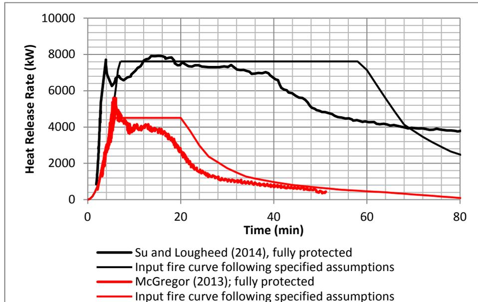
Figure 4-1: Heat release rate corresponding to the movable fire load
