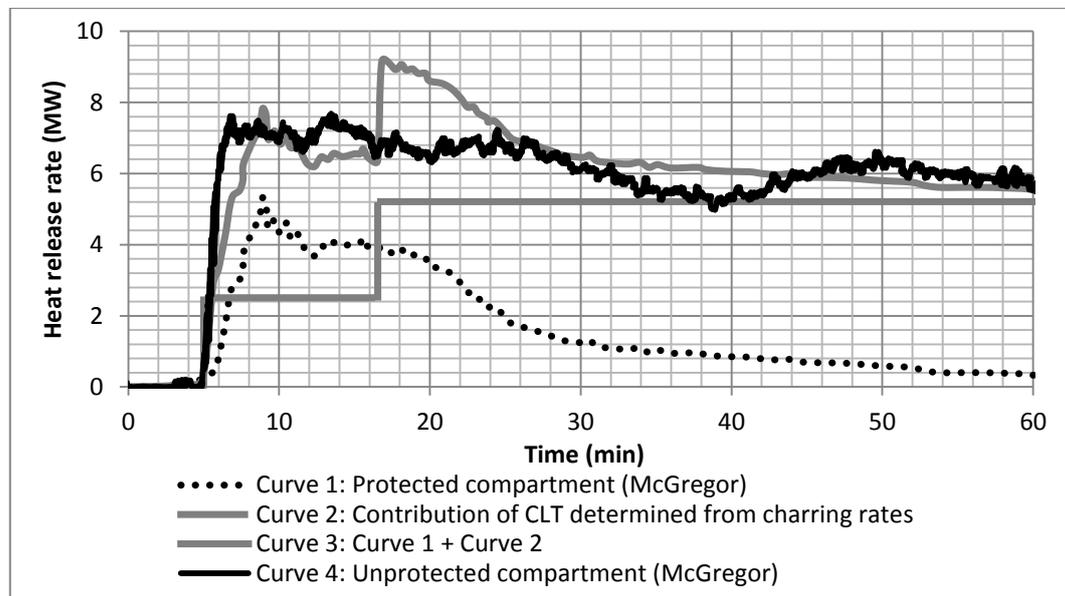
**Figure 3-2: Experimentally determined and predicted heat release rates in accordance with assumptions**
