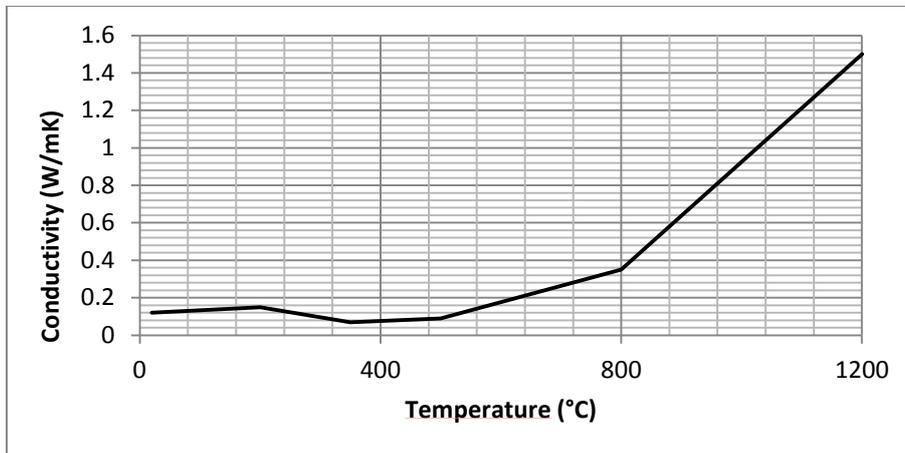
Figure 3-6: Effective properties for conductivity according to König and Walleij (2000)
