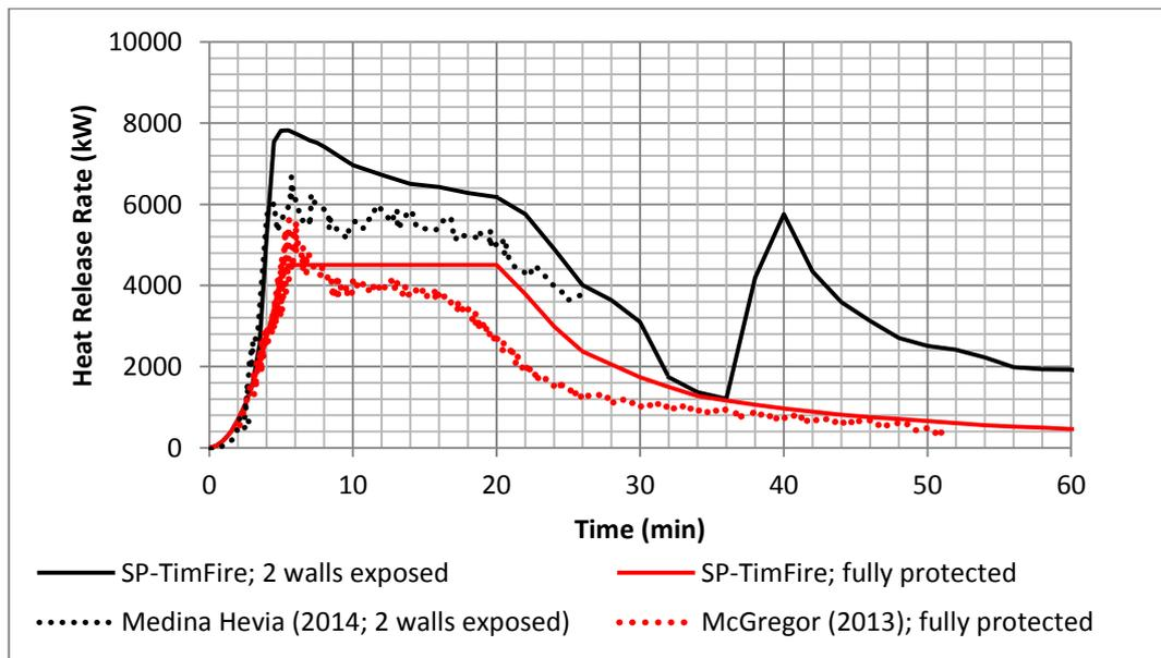
Figure 4-5: Experimental results and predictions using SP-TimFire for a fully protected compartment and a compartment with two exposed walls
