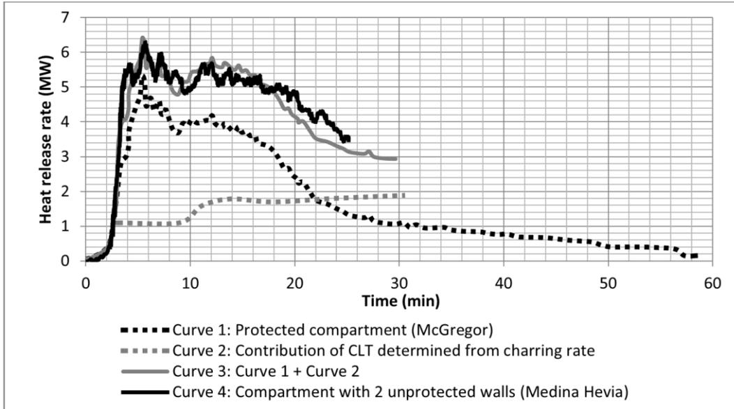
Figure 3-3: Experimentally determined and predicted heat release rates in accordance with assumptions
