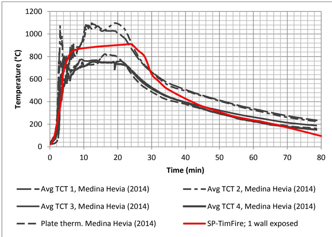
Figure 4-6: Experimentally determined and predicted temperatures for a compartment with one exposed CLT wall using SP-TimFire
