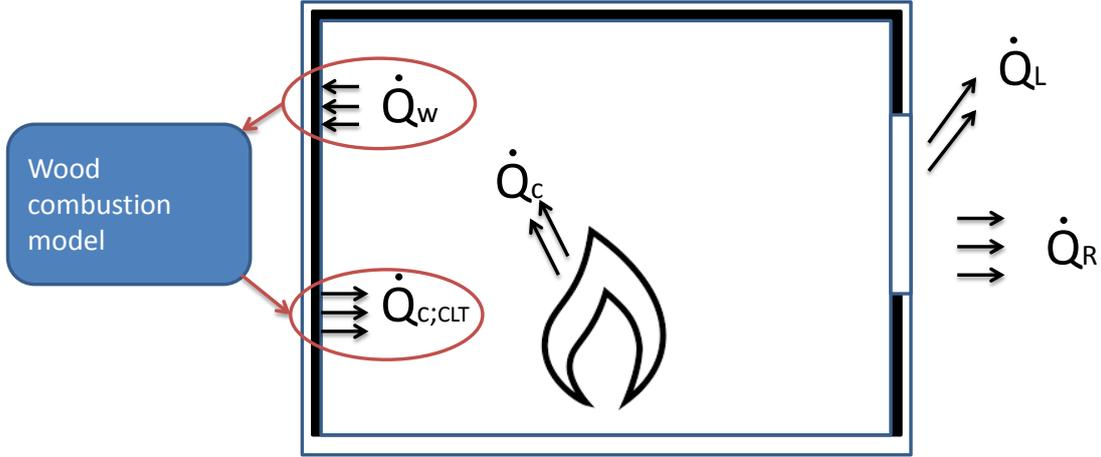
Figure 3-4: Schematic representation of SP-TimFire
