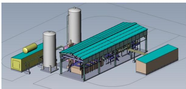
**Figure 4:** Overview of the complete facility. The left most building is the primary standard, next to it are the LNG and LIN storage tanks. The building in the middle contains the meter runs as well as the master meters and working standards (Figure 5 gives a close up). The building on the right is the control room.
