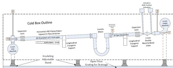
**Figure 6:** Sketch of the installation of one Master Meter within the Master Meter cold box. The whole line is slightly inclined to avoid entrapped gas pockets. The u-shaped object is the Coriolis flow meter, the brown boxes within the cold box are temperature transmitters whereas the brown boxes outside the cold box are pressure transmitters.
