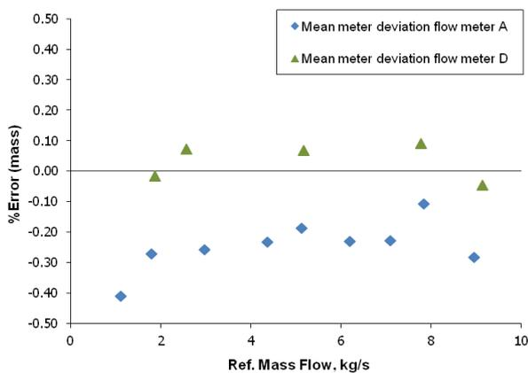
Figure 2: All meter deviations for meters calibrated with Liquid Nitrogen (LIN).
