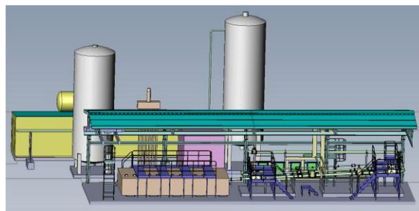
**Figure 5:** Master Meter Cold Box, The MuT meter runs, master meters and working standards. The Master meters are installed in a cold box (brown box on the left). The MuT meter runs are to the right of the cold box.
