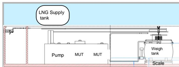
**Figure 7:** Sketch of the primary standard. Traceability is through the gravimetric method, hence LNG is pumped from the supply tank (top) through the MUT and then to the weighed tank (right).
