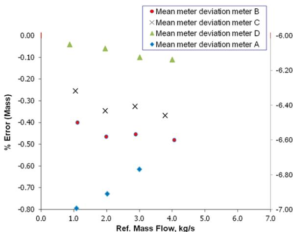
Figure 3: All meter deviations for meters calibrated LNG. Deviations for flow meter A are shown on the right axis. The errors for meters B, C and D are given on the left axis, the error for meter A is given on the right axis.
