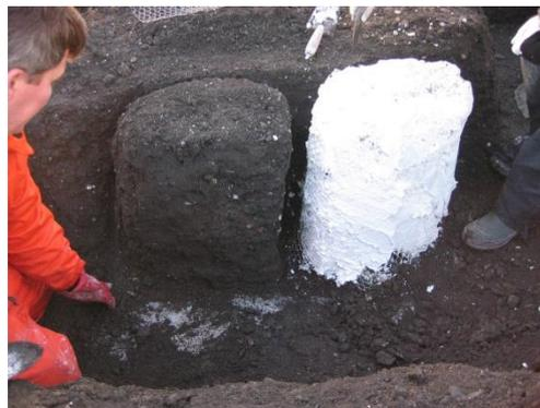
Figure 1. Sampling of in-situ specimens of bottom ash using mesh and gypsum.
