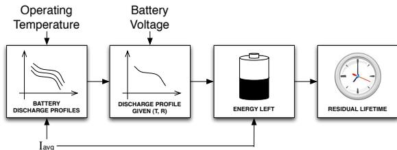
Fig. 8. Computing a node's residual lifetime.
