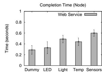
**Figure 3:** The completion times of RESTful web service calls on a Tmote Sky is well below one second.
