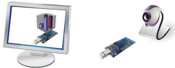
**Figure 1: Sensor data is displayed overlaid over the sensor itself, as captured from the live camera feed. Sensor data is queried from the low-power IP sensor network using a RESTful web service architecture.**
