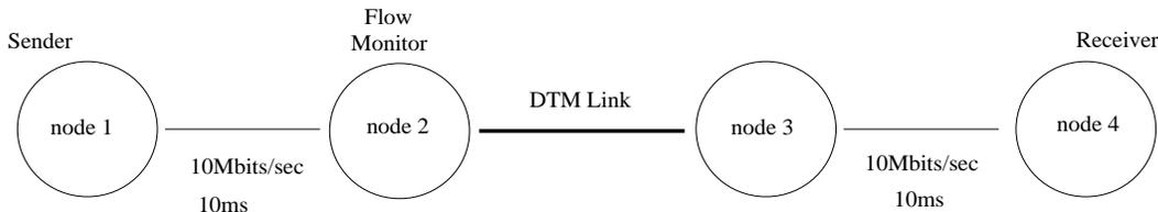
Figure 2: Basic Simulation Topology
