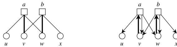
Fig. 8. The right-hand side shows the directed graph \vec{G} for the graph G and the matching M on the left-hand side. Observe how the alternating path p = [w, b, v, a, u] in G translates to a directed path in \vec{G} .
