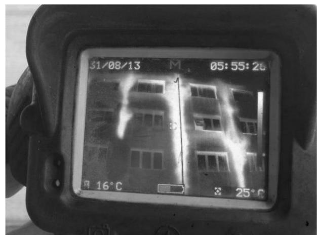
**Figure 9:** Fire spread through the cavities between the timber modules. Fire in Luleå 2013.
