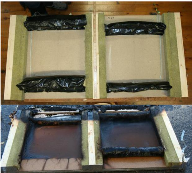
**Figure 11:** Fire barriers tested in the model scale furnace at SP. Before and after the fire test.
