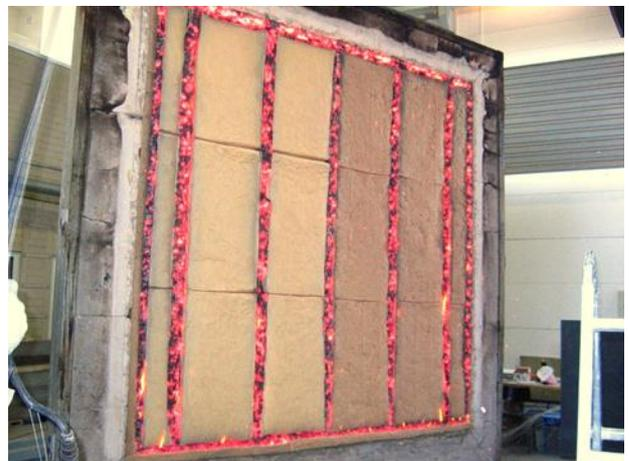
**Figure 13:** Mineral wool fixed using over-dimensioning after 60 minutes fire test.
