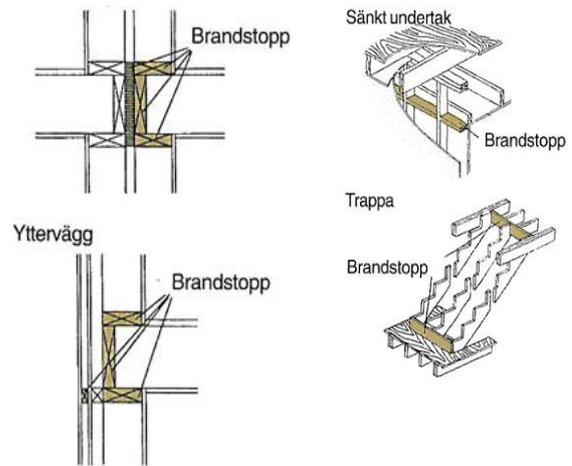
**Figure 12:** Detailing of fire stops can be only controlled at the building time [7].
