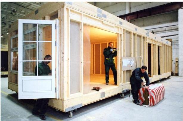
**Figure 7:** *A compartment for a modular building.*
