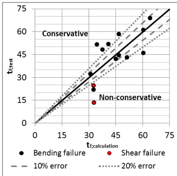
Figure 4: Test results versus predictions of the fire resistance using the 5<sup>th</sup> percentile strength
