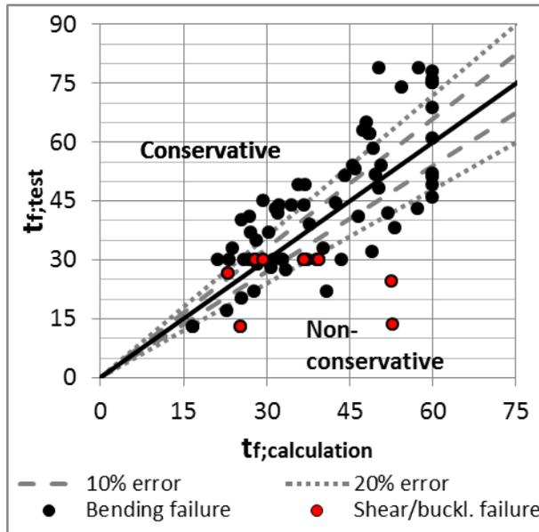
Figure 10: Test results versus predictions of the fire resistance using the **estimated strength**;
