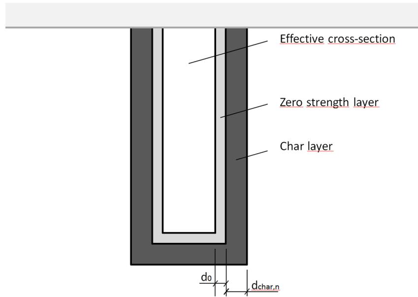
Figure 1: Effective cross section of a beam in accordance with the reduced cross-section method
