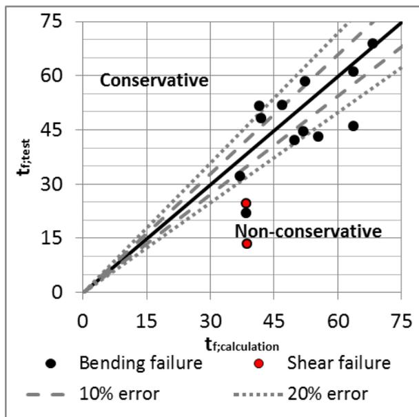
Figure 2: Test results versus predictions the fire resistance using Eurocode 5
