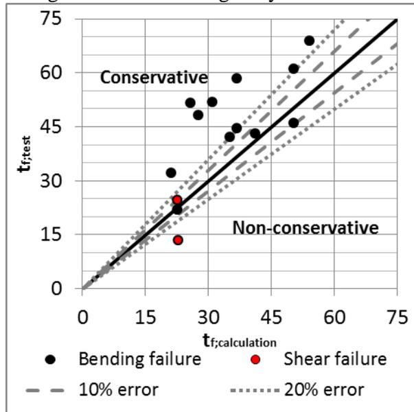
Figure 6: Test results versus predictions of the fire resistance using the 5<sup>th</sup> percentile strength and a doubled zero strength layer
