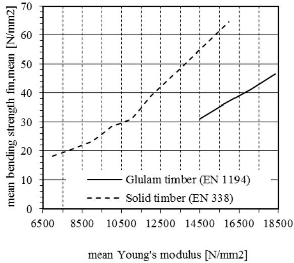
Figure 8: Relationship between the mean Young's modulus and the mean bending strength, according to the Probabilistic Model Code (JCSS, 2007)
