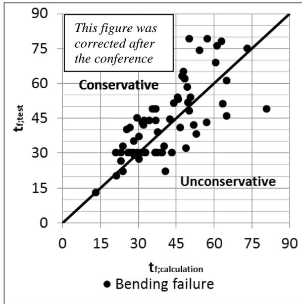
Figure 12: Test results versus predictions of the fire resistance using the **estimated strength**;
