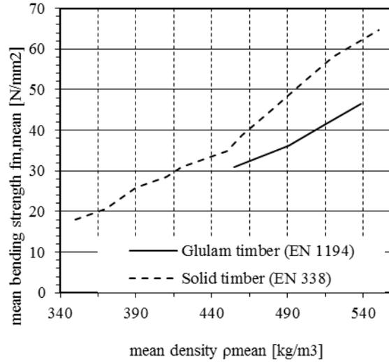
Figure 9: Relationship between the mean density and the mean bending strength, according to Probabilistic Model Code (JCSS, 2007)
