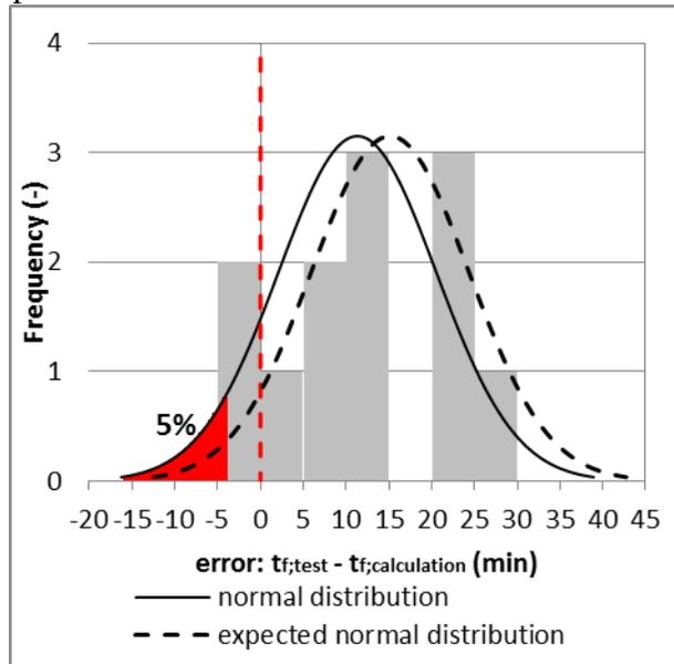
Figure 7: Frequency of errors and the corresponding normal distribution using the RCSM, the 5<sup>th</sup> percentile strength, and a doubled zero strength layer (bending failure only)
