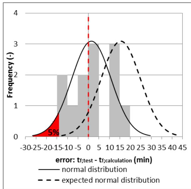
Figure 5: Frequency of errors and the corresponding normal distribution using the RCSM and the 5<sup>th</sup> percentile strength (bending failure only)
