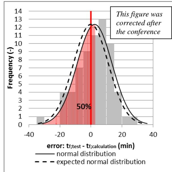
Figure 13: Frequency of errors and the corresponding normal distribution using the RCSM and the **estimated strength**;
