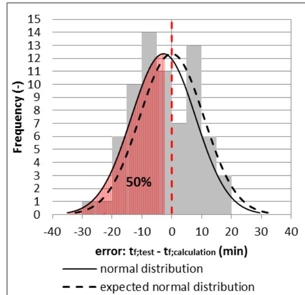
Figure 11: Frequency of errors and the corresponding normal distribution using the RCSM and the **estimated strength**;
