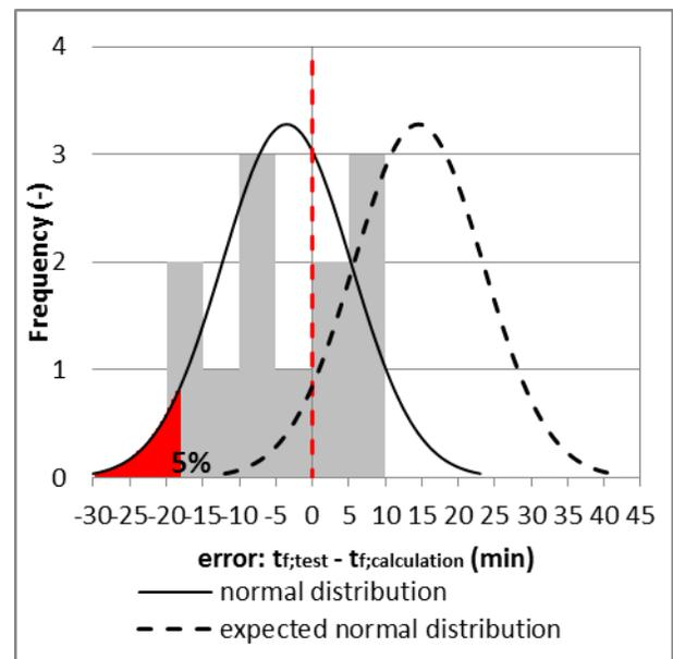
Figure 3: Frequency of errors, corresponding normal distribution and expected normal distribution using Eurocode 5 (bending failure only)
