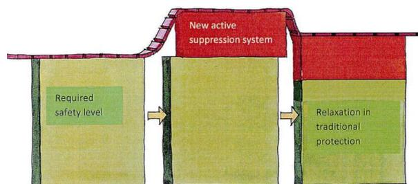
**Figure 3:** Principle for fire safety design by sprinklers: Increased fire safety by installation of sprinklers may lead to relaxations in the passive fire protection features, and still fulfil the same or higher safety level [23].
