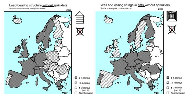
**Figure 1:** Restricted use of timber structures and visible wood set by national prescriptive regulations [1, 2]. Dark colours indicate that  $\geq 5$  storeys are allowed.
